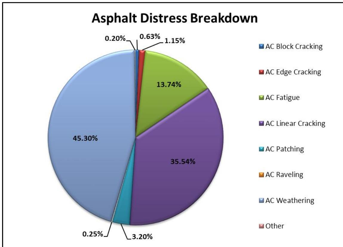
Figure 12: Asphalt Distress Breakdown
